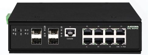
L2 Managed Lite Industrial PoE switch 8\*10/100/1000Base-T (RJ45 IEEE802.3af/at PoE) + 4\*1000Base-X (SFP) Ports
